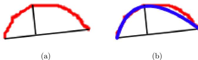
Figure 5-13: (a) A curved stroke with an illustration of the arc recognizer’s geometry calculations, and (b) the resulting smooth curve overlaid.
