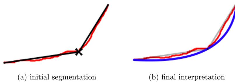
Figure 5-16: The (a) initial and (b) final recognition of what seemed to be two straight segments.
