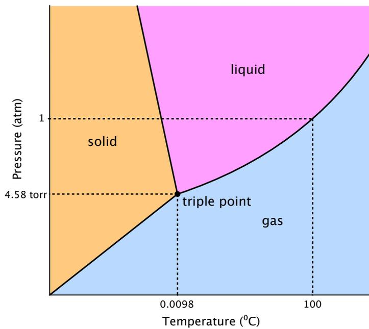
Figure 6-2: A user-created chemistry diagram showing the phases of water.
